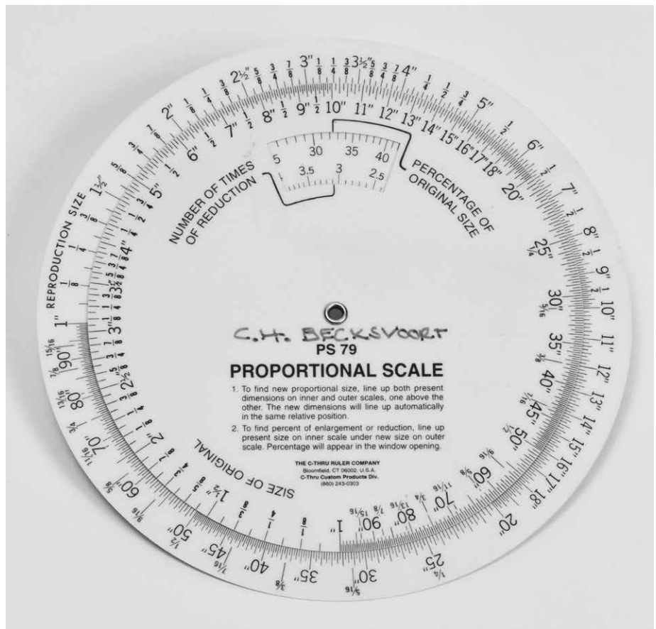
5-8. Architect's or Designer's proportional scale. This tool helps you determine the percentage of increase or decrease working from a specific size.
