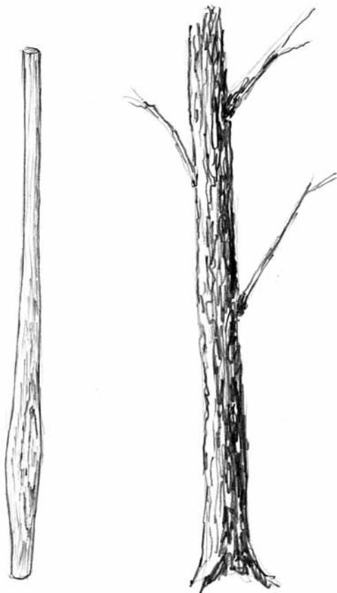
Parts split and shaved along their long fibers retain the strength of the tree.
