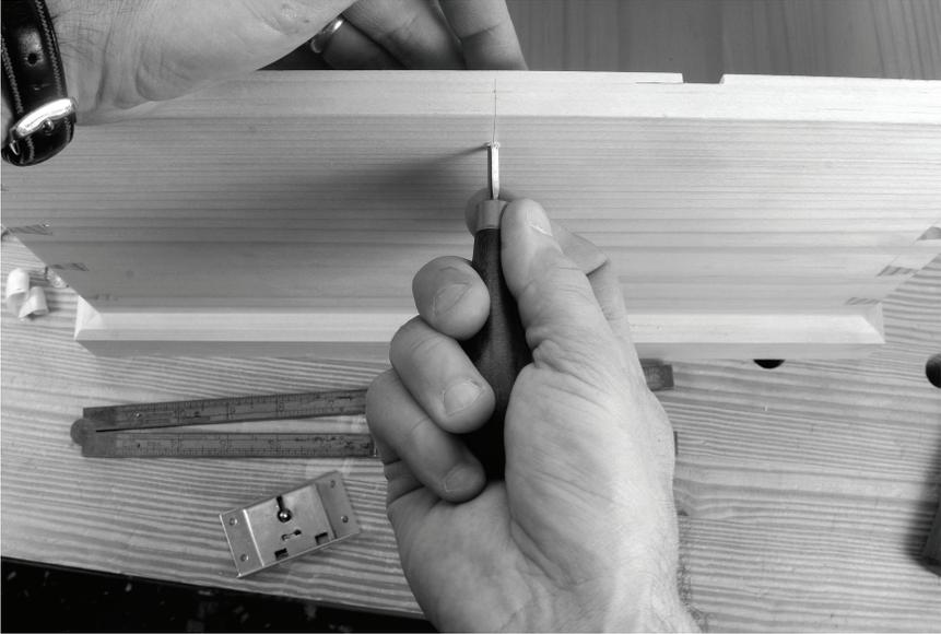
*Bore a hole through the front of the box using a birdcage awl. The sharp arrises of the awl will bore through the front. Barring that, drill a hole that is smaller than the pin in the lockset and test the fit.*
